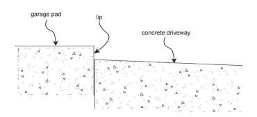
Make cuts parallel to the garage door opening with a cut-off saw at approximately 18" to 36" from the opening. The width will vary based on the concrete slope, hardscape height, border paver width (or length), DRiBOND° height, transition area and height of the slab being tied into. Create a smooth transition based on this information. Maintain slope away from the garage door opening or consider a french (deco) drain to divert water away from garage.
