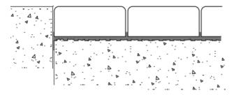
When ready in the installation process, mix the required amount of DRiBOND® with water and neatly trowel into the transition area as required. Proceed to lay the field/border pavers at the transition area, as well as tamping and leveling them lightly to the desired slope, seamlessly creating a smooth transition.
