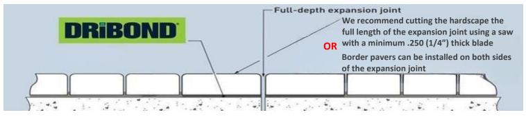
Of critical importance in freeze/thaw zones, overlaid hardscape materials must be cut with a wet-cut floor saw following the length of a full-depth expansion joint at 1/4" width or wider after DRiBOND® comes to final set after a minimum 6 hours. Alternatively, expansion joints can be left exposed by laying border pavers along each side of each expansion joint in such a manner that the expansion joint is not covered.
