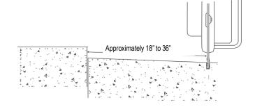
Start by making the first cuts at a depth of 3/8" at the furthest point away from the opening, and make progressively deeper parallel cuts as you get closer to the opening, where the final cut will be to the depth required to make for a smooth, weatherproof transition. The number of parallel cuts that must be made will depend on the height of the lip, and the distance from the transition area into the garage to where the first cut is made.
