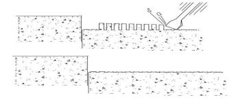
Once all cuts have been completed, you will need to utilize a chipping hammer with chisel to remove the concrete between cuts. Gently chisel away the concrete at the cuts closest to the garage door transition lip. Remove all chiseled concrete. A rough surface is O.K.
